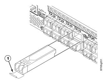
Figure 42. Replacing an optical transceiver
